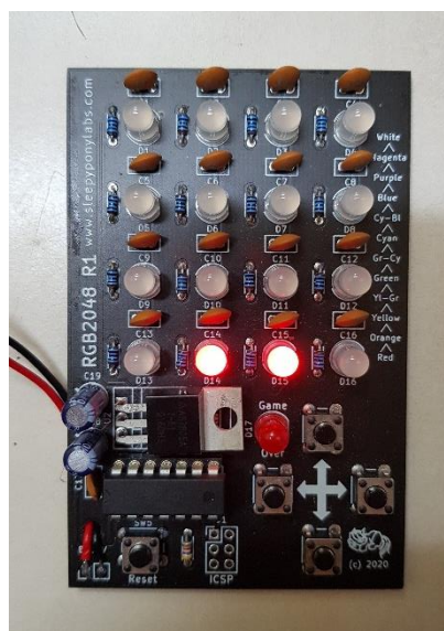
Two red LEDs lights up (correct power-on behavior)
